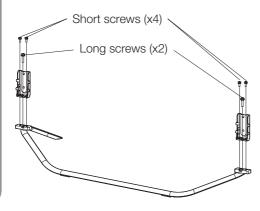
Place the TV on a flat surface with soft cushion on top of it. Insert the stand unit into the slot on the bottom of the TV while holding the stand unit to avoid it falling over.
