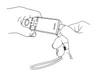
Figure 3: Pull the handle rope with your middle and index fingers and use your thumb to open the battery cover.
