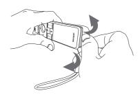
**3** Close the battery cover. Close the battery cover from top to bottom.
